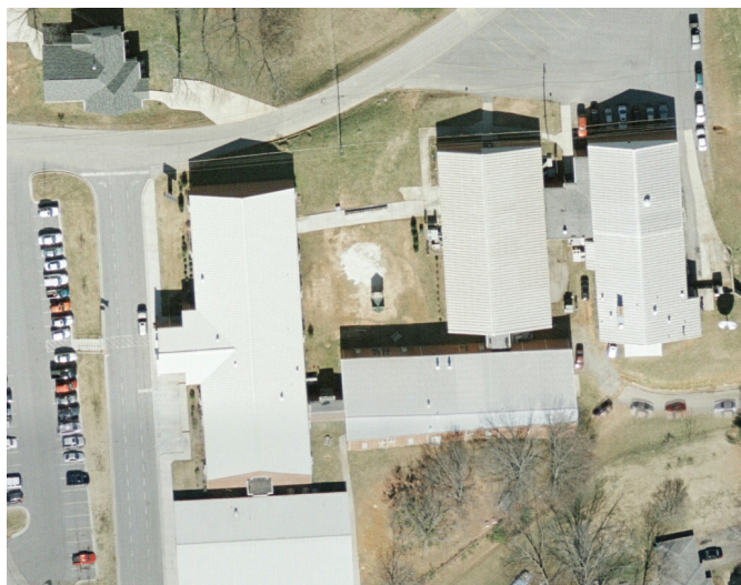
Compress choosing from more than 130 image formats. This true color example is an uncompressed GeoTIFF image with 6-inch (15.2cm) pixel resolution and an 8-bit radiometric resolution.
