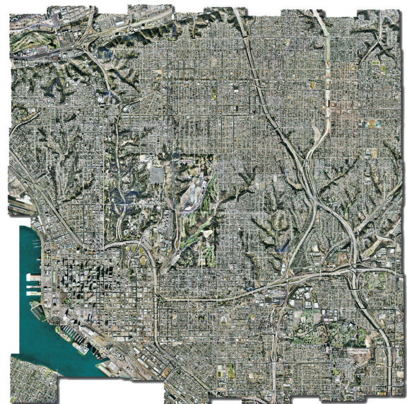
Before and After Before mosaicking and compression: Multiple images and 10GB of data After: 1 Image and only 500MB of data
