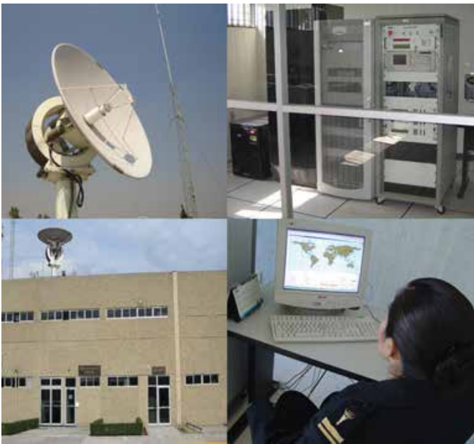
The Mexican Navy is responsible for operation of the Mexican SPOT Ground Antenna (ERMEXS), which is an advanced terminal for the reception, storage, extraction, and archiving of SPOT imagery.
