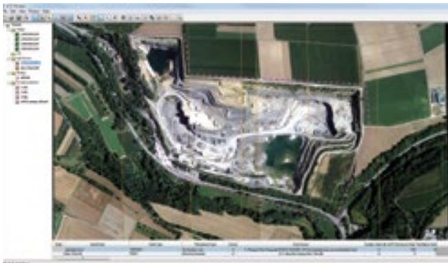
The pixel-by-pixel, multi-ray Dense Matching in IMAGINE Auto DTM can create highly accurate RGB-encoded point clouds directly from stereo imagery.
