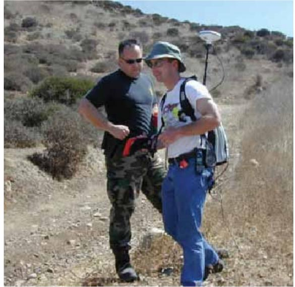
Greg Pendleton, Leica Geosystems, GPS, is collecting a ground control point. US Border Patrol Agent Daniel Isenberg is assisting.
